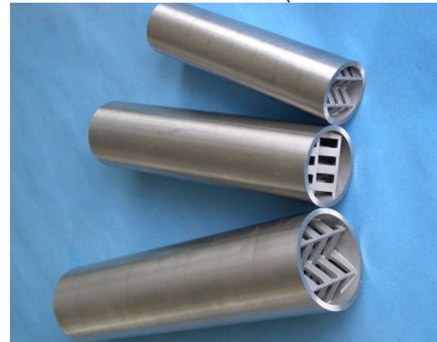
Mixing elements brazed together in a vacuum stove.
