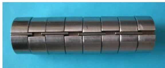
Picture 3: Assembly of eight (8) SMB-R mixing elements
