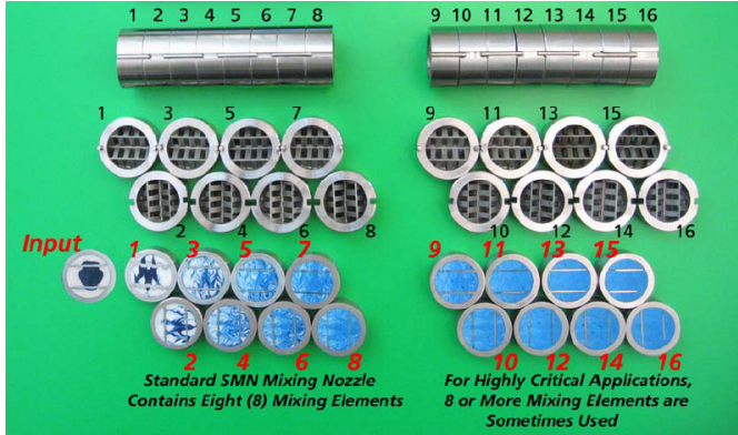
Fig. #4: Mixing evolution through the SMB-R Static Mixer Elements of a Blue and White resins (1:1 volumetric ratio). After 8 elements 80% and after 16 elements 97% mixing efficiency is achieved.
