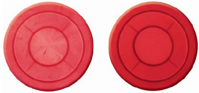
Fig. #5: Reduction of colour concentrate additives of as much as 30% can be achieved with comparable part colour density
