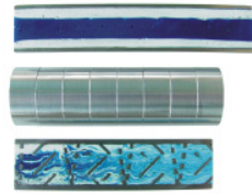
Mixing of epoxy resins in an empty pipe and in an mixer LMXR
